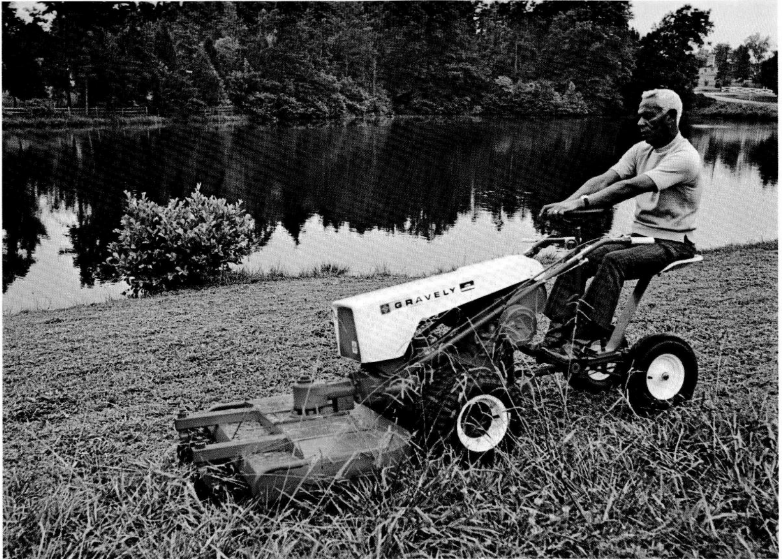
Gravely 7.6 Super Convertible with Optional Dual Wheels, Steering Sulky, and 40-inch Commercial Rotary Mower
